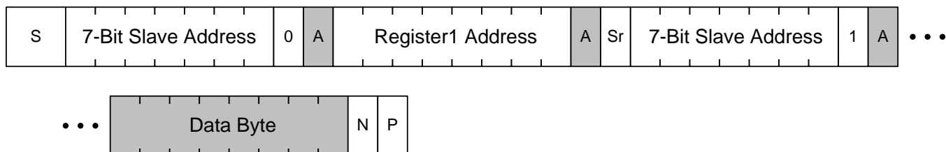
Figure 35. I 2 C Write Data Format
