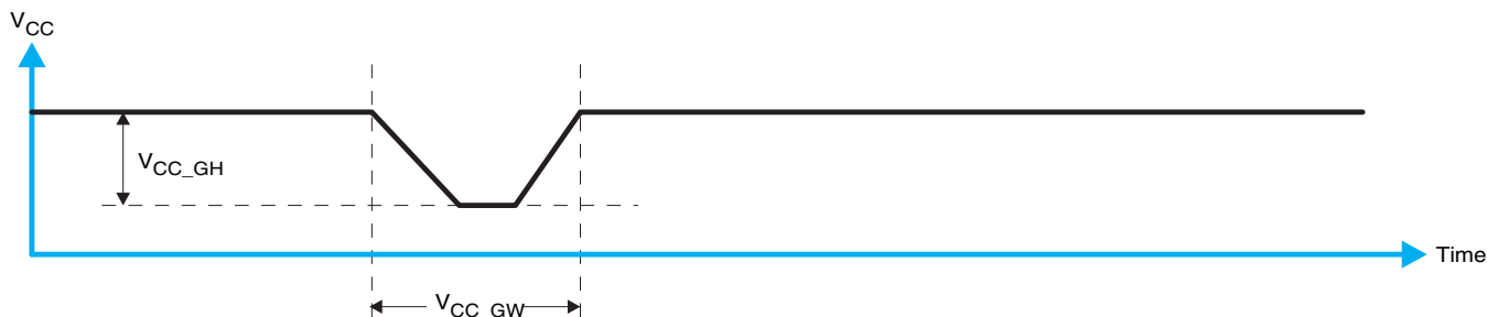
Figure 36. Glitch Width and Glitch Height
